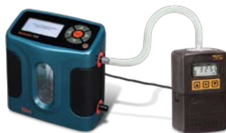
AirChek 2000 and Defender in CalChek calibration train
