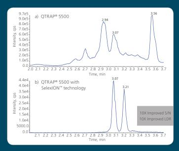
Injection of clenbuterol at 5 pg/uL in urine: (a) High chemical noise makes the detection impossible. (b) Differential ion mobility separation (DMS) increases selectivity and eliminates the high background producing a 10X improvement in signal-to-noise.
