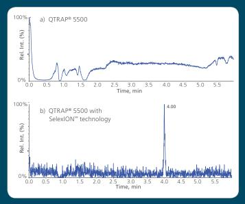
1pg/uL injection of Pentoxifylline in plasma: (a) High chemical noise makes the detection impossible. (b) Differential mobilirt separation (DMS) increases selectivity and eliminates the background.
