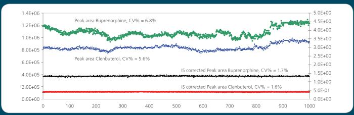
The above figure of 1000 injections of spiked Buprenorphine and Clenbuterol in protein precipitated human plasma demonstrates the unique reproducibility, robustness and stability of the SelexION™ technology in combination with the SCIEX QTRAP® 5500 System. A total of 66 hours of consecutive analysis produced a % CV of less than 7% in the peak area for both Ruprenorphine and Clenbuterol.
