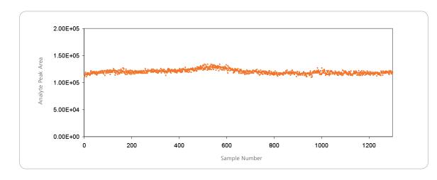
The very low % CV of 3.3 for the analyte peak area of 1300 injections of spiked Diazepam in protein-precipitated human plasma demonstrates the industry-leading ruggedness, reproducibility and reliability of the QTRAP® 5500 System.
