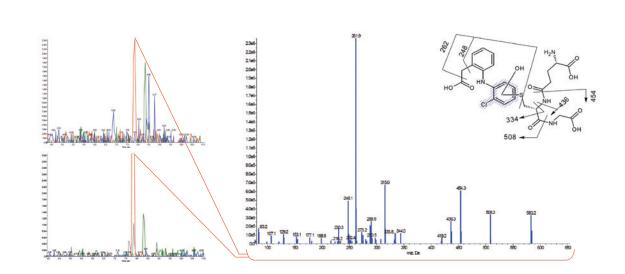
The power of TripleTrap™ scanning is illustrated in the above metabolite ID example. In this UHPLC experiment, two survey scans for characteristic GSH fragments, a positive ion neutral loss of m/z 129 and a negative ion precursor ion scan of m/z 272, automatically trigger enhanced product ion scans to screen for potential reactive metabolites. Including the polarity switch between survey scans, the total cycle time is 2.1 seconds.
