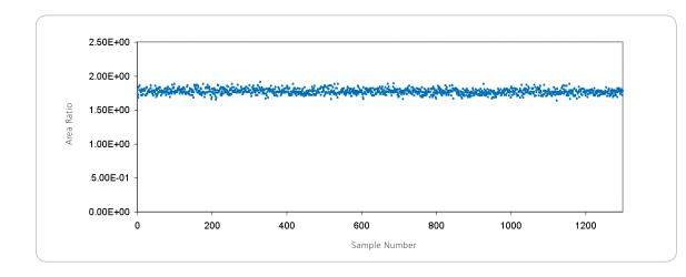
The excellent % CV of 2.3 for the area ratio of Diazepam and deuterated internal standard in protein-precipitated human plasma shows the reproducibility and stability of the AcQuRate™ pulse counting detector for consistent quantitification results day in day out, week after week, month after month.
