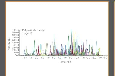
With dwell times as low as 1ms, the 4500 series is ideally suited for multi component contaminant analysis as these data demonstrate with the detection of over 200 pesticides at 1ng/mL. The faster electronics and the intelligent *Scheduled* MRM (sMRM), permits the screening of hundreds of pesticides in a UHPLC time scale.
