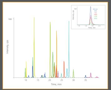
Highly multiplexed peptide quantitation using the Scheduled MRM<sup>™</sup> algorithm. 30 selected MRM transitions from a 4000 MRM assay of tryptic peptides. This experiment was run in replicate on an Eksigent 200 um ID cHiPLC<sup>®</sup> column with peak area deviation < 10%. Insert: an example of multiple MRMs to a single peptide, showing selected fragment ion chromatograms.
