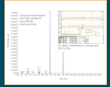
Combining intelligent peak detection with the ability to trap and scan out ions on a UHPLC time scale, creates a potent solution for detecting unexpected contaminants. Add to this a single library of thousands of QTRAP spectra for library matching, and contaminants at the lowest levels can be confidently identified.
