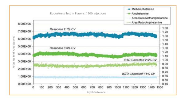
The excellent reproducibility for the peak area ratio of Methamphetamine and Amphetamine in human plasma shows the stability of the AcQuRate<sup>™</sup> pulse counting detector for consistent quantification
