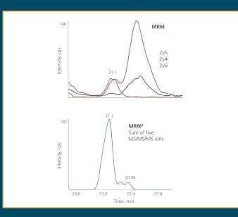
Quantitation of tryptic peptides in a complex matrix. Higher selectivity workflows such as MRM<sup>3</sup> (bottom) can provide additional specificity for low level detection of compounds when high background or interferences render MRM workflows ineffective (top).
