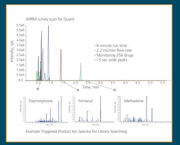
The QTRAP 4500 system allows *Scheduled* MRM (sMRM) to trigger high quality, full scan product ion spectra for use in library searching. With highly sensitive Triple Trap<sup>™</sup> scanning it is possible to confidently identify compounds at up to 100X lower concentrations than triple quadrupole full scans.
