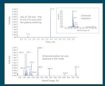
Troglitazone GSH adduct was detected using complimentary positive neutral loss and negative precursor ion scans, combined with Information Dependent Acquisition (IDA) linear ion trap scans. This unique workflow results in the comprehensive detection and characterization of GSH adducts in a single injection
